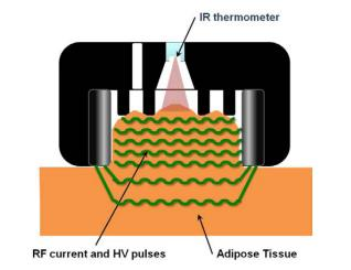
Figure 1: The TiteFX hand demonstrating RF current passing between the electrodes through the adipose tissue in the suction cavity and down into the subcutaneous tissue.
